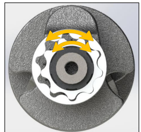
Excessive torsional vibration 'rattles' gerotors during operation creating high impact forces - further increasing contact loads
